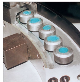
Adjustable bearing design
